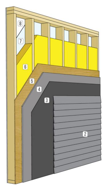
Therefore, the proposed wall assembly theoretically meets and exceeds the minimum requirements of RSI 2.97/R16.8.1 RSI = R = 1.67826
